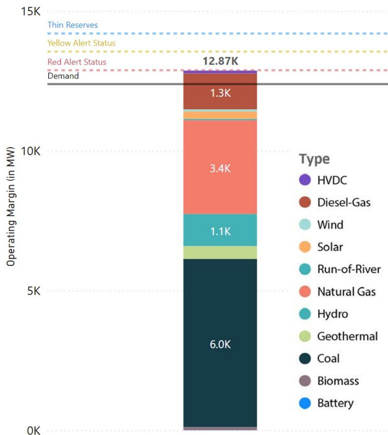
The lines indicate the demand (black), and reserve statuses. The stacked bar represents the computed power supply (in MW) for this period given the assumptions of this scenario.
