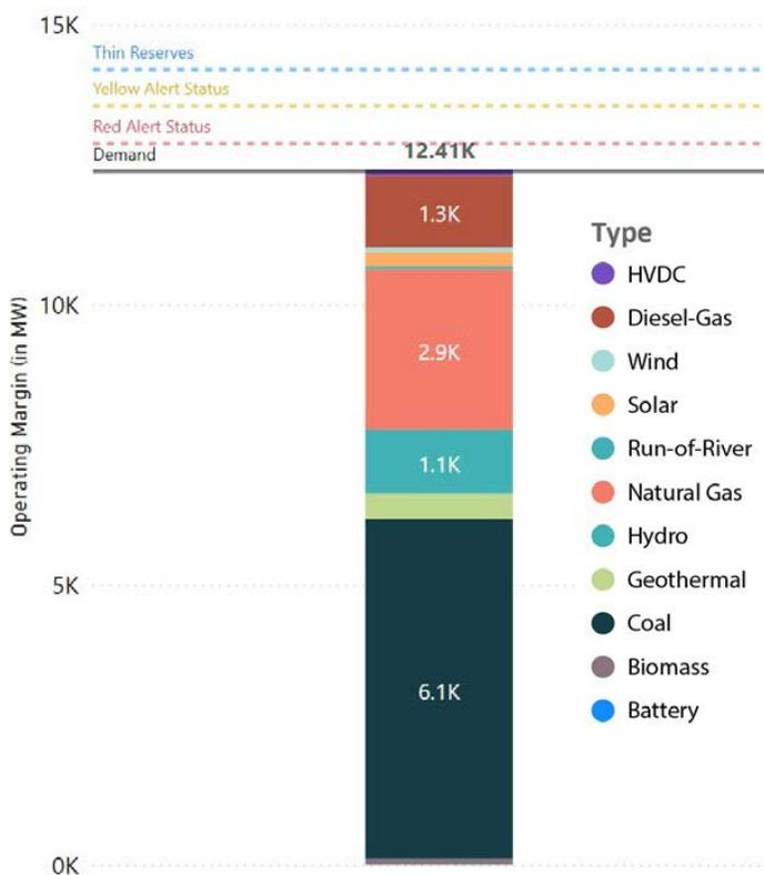
The lines indicate the demand (black), and reserve statuses. The stacked bar represents the computed power supply (in MW) for this period given the assumptions of this scenario.
